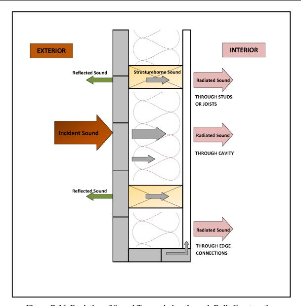
Figure B-16. Depiction of Sound Transmission through Built Construction
