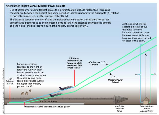
Figure 3-1. Afterburner Takeoff versus Military Power Takeoff
